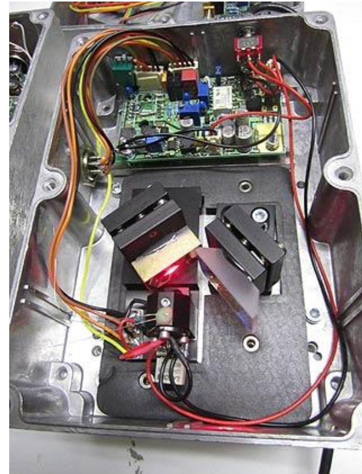
Fig. 1. (Color online) Schematic of a Littrow configuration ECDL
